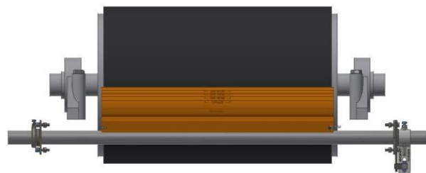
Fig. 3b Cleaner centred to the pulley
