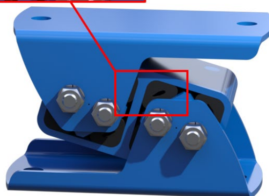
Damaged suspension unit – reduced height, cracking / hollowing of rubber components
