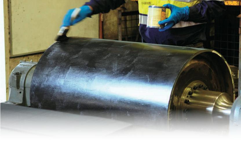
Our range of rubber and polyurethane lagging is designed to be applied on any pulley. Strip lagging is cold bonded to the pulley shell and can be applied either in-situ or within a workshop envrionment. The lagging comes in a 250mm wide strip and has a fully vulcanised CN bonding layer ensuring a rubber tear bond to the pulley shell. This lagging is available in both Natural and Fire Resistant Anti-Static (FRAS) rubber and polyurethane.
